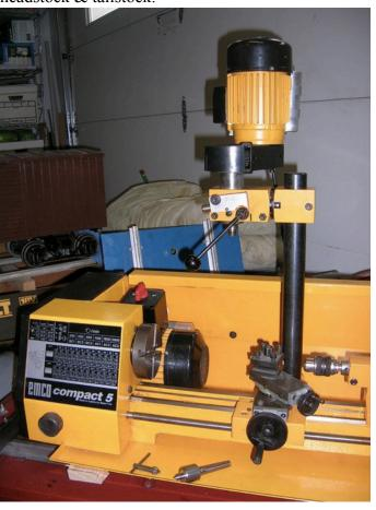
The vertical milling & drilling unit is included and converts the lathe into a complete mill/drill unit. The milling/drilling head is equipped to accept the supplied drill chuck, has a vertical fine-feed attachment and is moveable in 3 dimensions. The belt between the two pulleys will need to be supplied.
