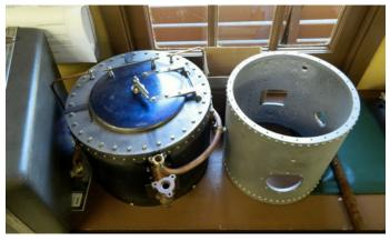
Jerry Kimberlin surpassed himself this month with a large collection of bits and pieces, including no less than two large-scale smokeboxes. The first was for the Heinz Atlantic. It had been riveted to the boiler shell, requiring the time consuming task of removing all of the rivets before it can be cleaned up and painted with a heat resistant coating.
