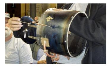
The second smokebox was an even more imposing piece of equipment, that Jerry has built, for the Garrett locomotive he has been working on for the last several years. For those not familiar with Garretts, they were articulated engines in which the boiler spans the space between the front and rear power units, supplying steam to both. On completion, this engine should be one of the most powerful in the Club!
