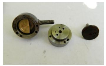
Anthony Duarte - Brake Cylinder Valve - His first effort was in Stainless steel, but due to the toughness of stainless steel, two taps were broken, which rendered the valve unusable As a result, a replacement made of brass was made to work.
