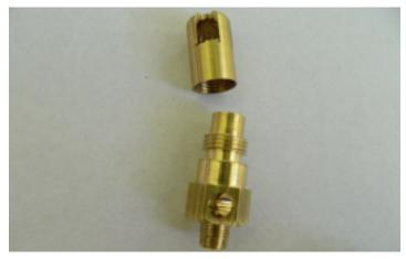
Jerry Kimberlin - Produced 24 brass burners for various projects, some of which were for the Heinz Atlantic. Photo shows a burner with a broken flame spreader head.
