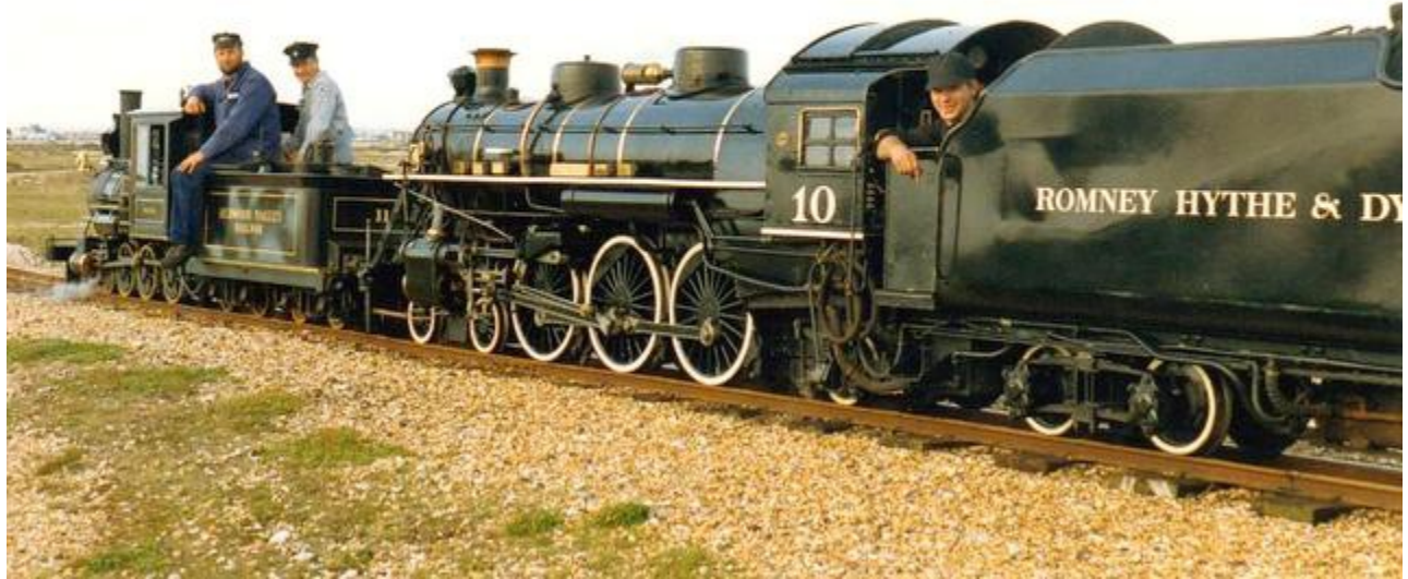
Here is Redwood Valley's #11 along with a 15" gauge 4-6-2. Pretty massive chunks of iron!
