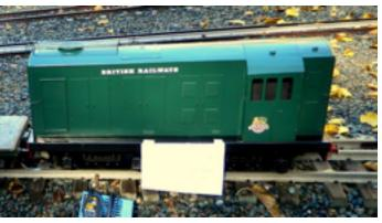
Two year old 1" scale, 4.75" gauge locomotive with wireless radio controlled system for control of speed, braking and pressure regulated dual tone air horn.
