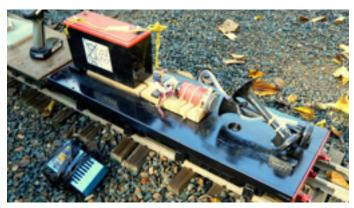
There are 4 motors where each axle are powered and it includes a new Extreme Racing 30 12v battery and trickle charger.
