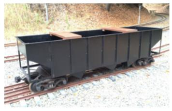
Three bay steel hopper car in very good condition with little running time. Car body and cast iron trucks by Tom Bee. Can be used as a riding car and/ or display car for your train.
