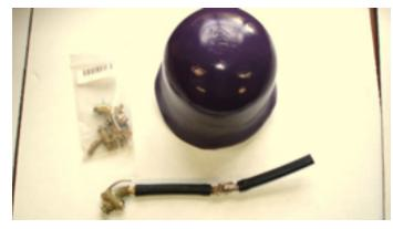
Working Air Fittings & Valves (Westinghouse design) where the glad hands are from Shapeways and he made the valves, each valve composed of 6 different components, 5 which were made from lost wax castings.
