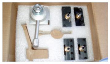
Mark Johnson – Tool holder set for a small lathe, similar to the Sherline line of tools, at a very low price (imported).
