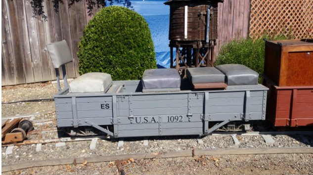
Riding car USA #1092, Narrow gauge, 5 feet long, 18" wide
