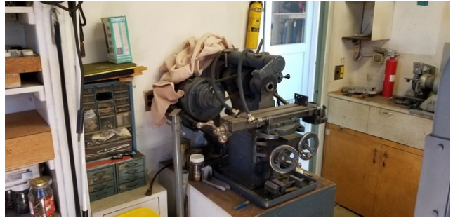
Burke Machine Tool Company, Model #126A horizontal bench mill
