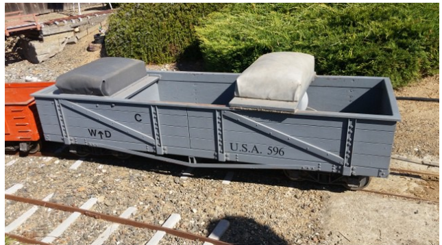
Riding car USA #596 Narrow gauge model, 5 feet long, 18" wide
