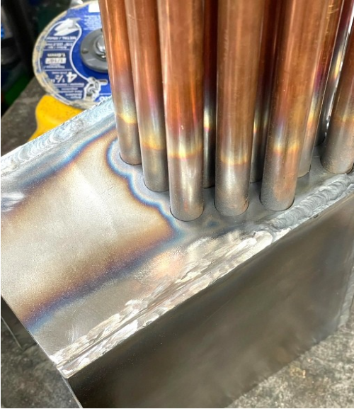
Copper flues attached the the firebox.
