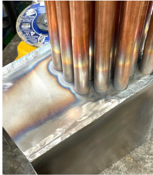
Copper flues attached the the firebox.
