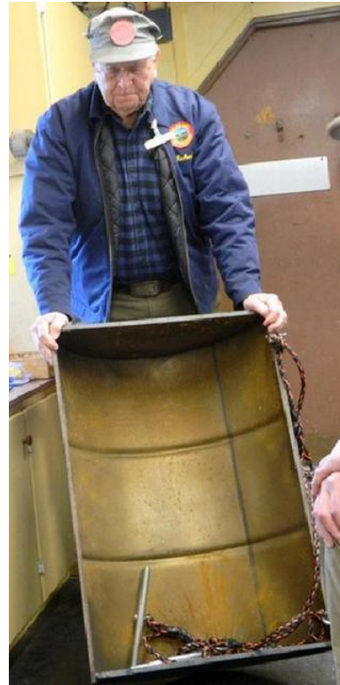
Rich Croll had a different kind of item to show this month. It is a tool for moving ballast gravel and is made from a light weight 55-gallon steel barrel. To provide additional edge support Rich fabricated and welded a rim made from \frac{1}{2} inch angle iron. So Rich, who's working on those freight cars while you're doing this kind of stuff?
