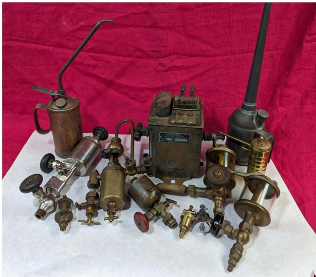
Prototypical lubrication systems. Oil cans, drip oilers, manual pumps, mechanical lubricator and a selection of oil & grease cups. The long spout is about another 11” tall.
