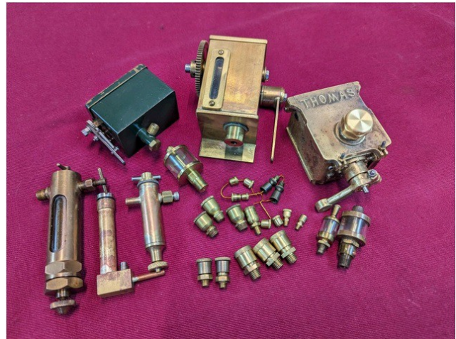
A group of scale lubrication devices: mechanical, displacement, oil & grease cups
