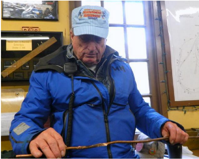
Paul Hirsh was solving a stuck check valve issue on the club's RG-22 locomotive when he noticed the copper water line between the axle pump and the boiler check valve was a little bit restricted.
