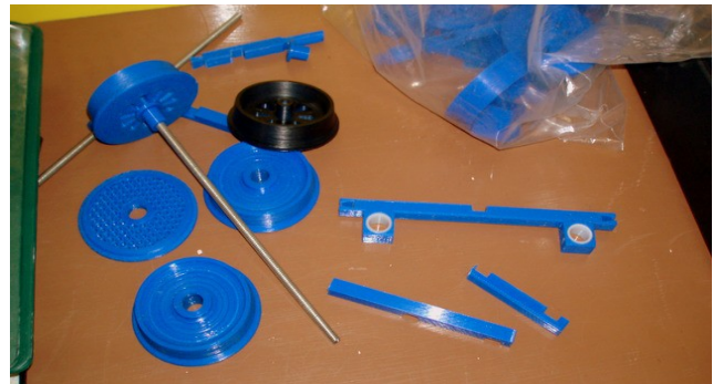
Dave August - Short presentation on "The Future" (of our Hobby). Sage advice from a long-time respected and self-taught member of our Club on the ever-increasing "simplicity" of our hobby. Showed us the results of "3D Printing" of locomotive parts, made from a material called PLA (Poly Lactic Acid), a type of plastic. Presumably, the procedures can be implemented onto metals, such as are utilized by our hobby.
