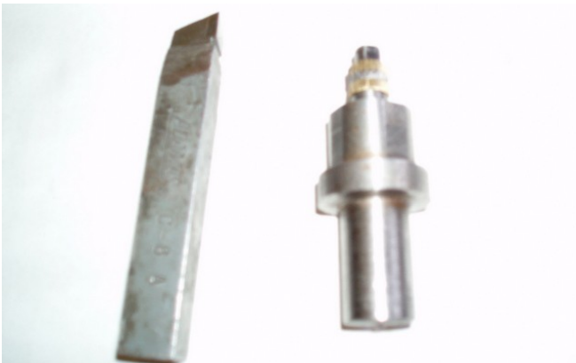
Jim Conover - A "failed" attempt at producing a ratchet wheel, presumably for use on a model-size lubricator. Nice effort at producing a mandrel to hold the ratchet "blank", but what is good about this experience is that fellow club members have workable solutions to offer, and in the atmosphere of the "Bits & Pieces" segment, potential problems can be solved by knowledgeable fellow members.
