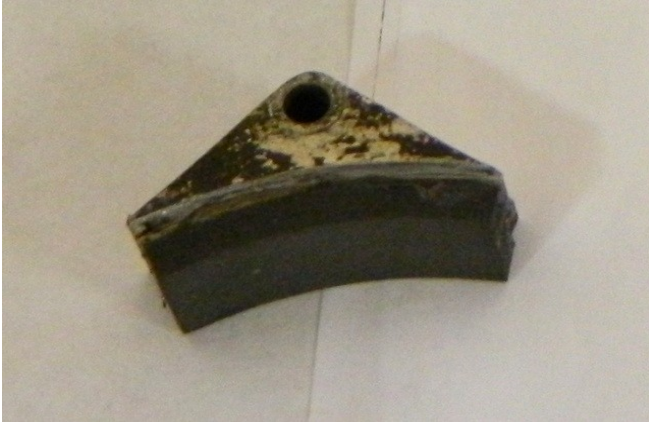
Rich Croll - A Home-fabbed Brake Shoe, made from Friction Material (that's what it's called!) purchased from McMaster Carr Industrial Supply house.
