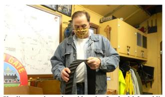
Charlie next showed a rubber tire for the McLaughlin tractor wheel made from a sheet 4 inches wide with treads cut on a radial arm saw. He fixtured the rubber sheet, clamped it down solidly, put a pair of dado sets together so he could make each groove in one pass, 3/4" wide & 3/16" deep. It smelled bad when do the individual cuts.
