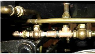
Using the lowest pipe, water from the steam pump comes in from the left or water from the injector comes in from the right; then it goes up and into the boiler.
