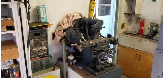
Burke Machine Tool Company, Model #126A horizontal bench mill
