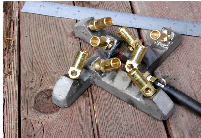
A home made 8 jet impinged burner with temporary gas connection for test.
