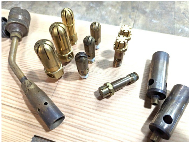
A group of barber jets, star & fan pattern. With a couple jet burners and a propane torch head as well.
