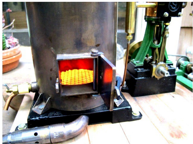
Here's a ceramic burner in a 4" diameter vertical boiler using a propane torch burner as a mixing system.
