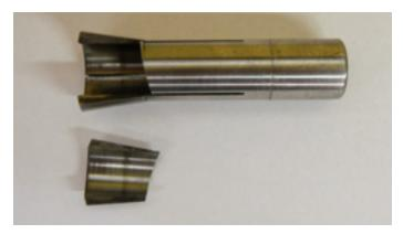
Rich Croll – Broken "R-8" Collet, a demonstration of how fragile some imported tools can be.
