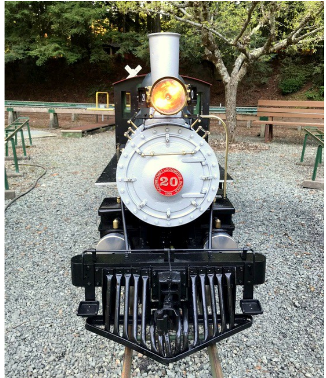
RG20 has had a clack on the right side, only when under light load. The rod bearing side play was measured to be up to 0.025", so it was assumed to be the source. Shims from Delrin were made to decrease the side-play to 0.005", but the clack is still there. So it goes with steam engines! Other potential sources will be investigated (cross slide?). Did I mention that this is a labor of love?
