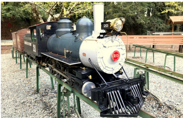
The RG20 repainting is almost done. The smoke box, stack, cylinders, steam chest covers and pilot have all been re-painted. The only tasks left is to repaint the running boards, cab top, and touch up the boiler cladding. Thanks to Bob Cohen for finding the original paint for the cladding.
