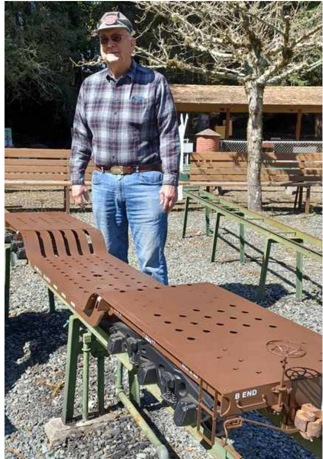
Richard Croll brought up his new depressed center 125-ton flat car with six-wheel Buckeye trucks. Another one of Rich's handsome projects!
