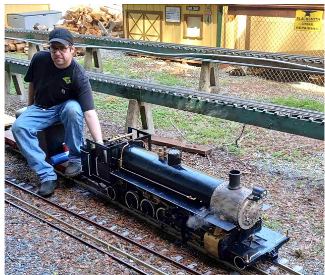
Evan Guinta steaming his 2-10-2T sans tank. Evan has been doing a wonderful job with this locomotive! An upcoming project will be building the saddle tank.
