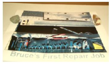
Bruce Anderson – Lessons learned while working on his locomotive, in the area of lubrication. Photo shows wear of metal parts caused by improper lubrication.
