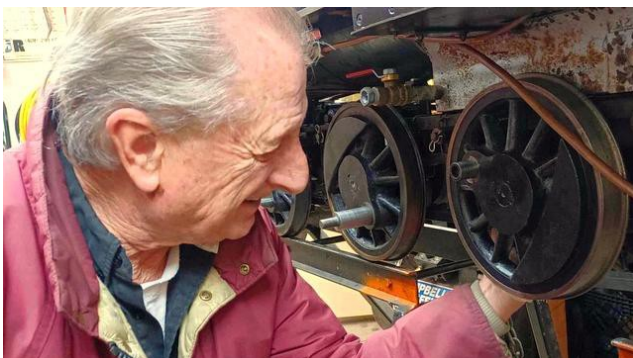
Paul Hirsh replaces a driver on the RG20. New tires were turned and assembled by Jerry Kimberlin.
