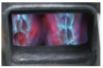
His third test was to go lower the burners to increase surface area — BINGO! He's still doing some tweaks with gas pressure and may add some firebrick but the engine is now making it around the track at 100 PSI.
