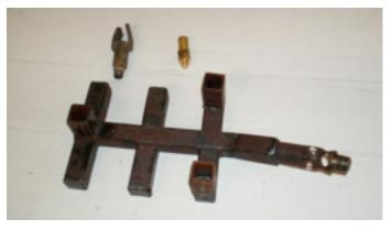
Bruce Anderson – Failed propane manifold burner (black assembly) for Harley, his 0-4-0T tank engine. Upper top left is a duckbill burner from a wok burner and the right is a wok impingement burner. See the accompany article in this newsletter on more details on Bruce's Saga.
