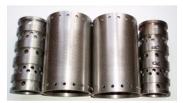
Rick Reaves – Cast Iron Cylinder Sleeves for Little Engines 0-6-0 Switcher.
