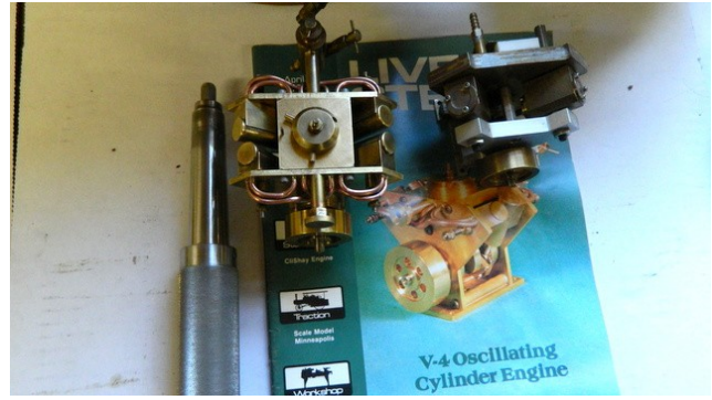
Charlie Reiter – Die holder with #3 Morse taper; small engines for R.C. boats inspired by articles in "Live Steam" magazine.
