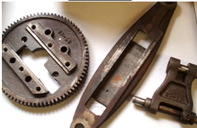
Anthony Rhodes – Cast Iron spare parts for an Atlas Shaper.
