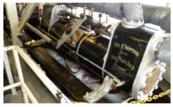
He had a chance to see the DUAL triple-expansion, horizontal 1925 steam engine up close, which was installed on the newly built 1971 riverboat.
