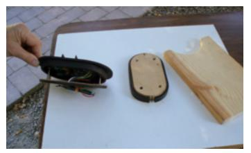
Dan Swanson: Forming Patterns for Sidewall/Signal Head. The patterns are made of wood, and the forming plate is MDFB. The Signal head is made of ABS plastic (TAP Plastics). The oval shape is produced by placing an ABS plastic strip in the oven at 270 degrees for a few minutes, which allows for approximately ten (10) seconds working time.
