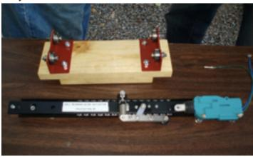
Steve Vitkovits: Actuator and Engine Test Stand. The Actuator utilizes a used drawer slide. The Test Stand (one unit for each pair of opposed drivers) has a wood base with roller bearings mounted on paired angle irons.
