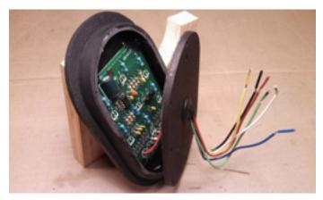
The signal body is constructed from a thicker, higher impact-rated ABS polymer and secured in place with stainless steel mounting screws. The display lights are ultra white 5mm long life 12 to 15 candle power LEDs and an interior sealed printed circuit board ensures operating reliability over time.
