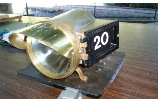
Bob Cohen: Headlight for GGLS Club Engine (under construction by Bob for GGLS). The headlight is made of soldered Brass materials (with the exception of the steel base), with a glass lens and reflector procured from a large commercial flashlight. Four (4) "AA" Batteries are contained within the headlight body.
