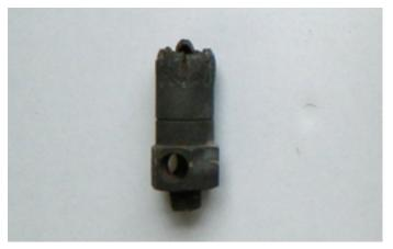
Rich Croll talked about the melted, burnt propane burner removed from one of the club engine's firebox burner manifold. Cause is unknown but the prevailing theory is that the burner was partially clogged which allowed the hot part of the flame to get too low.
