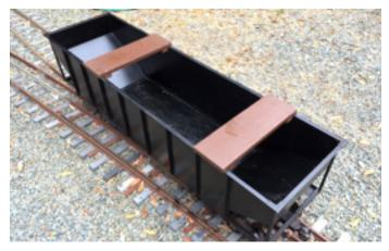
Detailed with optional ribs welded onto car sides. Ends have been reinforced for the included safety chain hardware.
