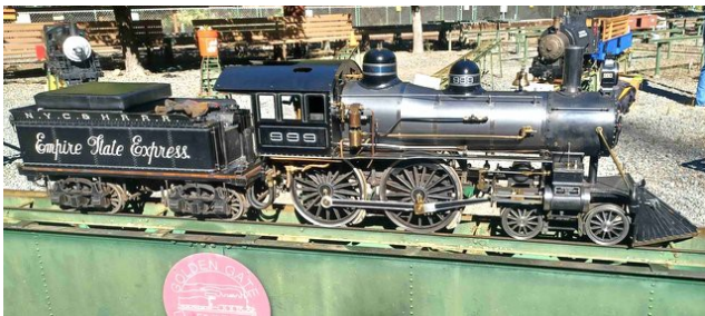
Charlie Reiter brought the 4-4-0 #999 "Empire State Express." Look at the size of those drivers.
