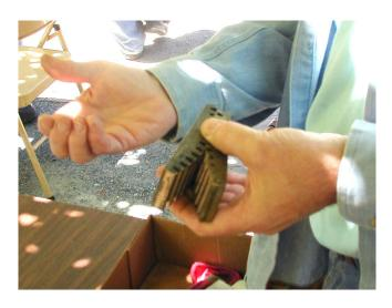
Charlie Reiter showed a pair of arc sections cut from a large (> 12") toothed gear. The sides opposite the teeth were machined flat and when the teeth of the two pieces were engaged, they formed an adjustable angle parallel for a large machine vise. A very clever tool salvaged from a large gear wheel.
