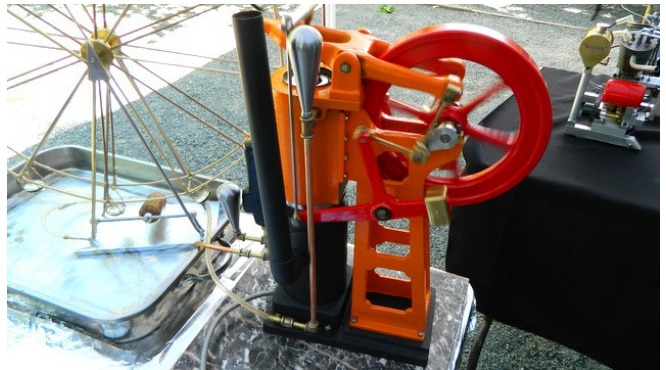
Model of the Improved Ericsson Engine by the American Mgm Co. driving the water wheel on the left.
