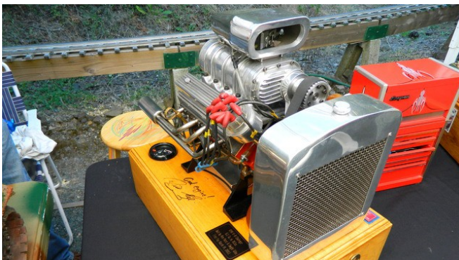
Patrick O'Connors' radiator showing hidden inside the engine stand box of Ken Hurst's Black Widow V8 engine.
