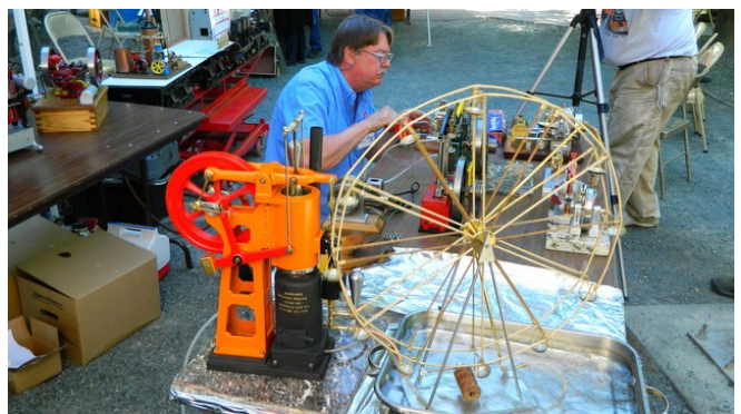
Model of the Improved Ericsson Engine by the American Mgm Co. driving the water wheel on the left.
