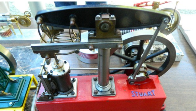
A nice looking Stuart walking beam stationary steam engine also built by Paul Denham.
