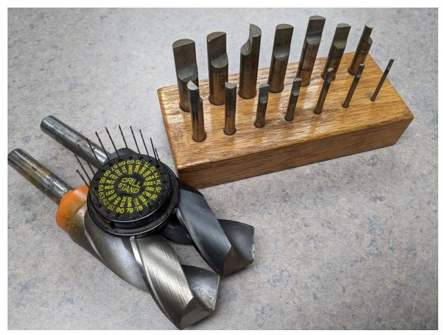
In this picture we get a closer view of "dee bits" which are great for making seats in check valves. These were commercially made but they are easy to make up as needed. The two "blacksmith" drills are 1.25" diameter. One is sharp, the other (orange) is dubbed. You can just see the little edge flat. On top of those is a set of twist drills from #61-#80. The range size in these tools is huge. Biggest twist drill I ever used was 2.5" diameter and the smallest .006".
