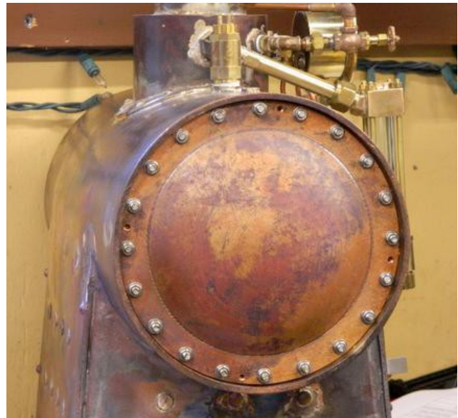
The boiler ends were shown during the October meeting and are secured with 20 studs & nuts and sealed with an O-ring. In full-size they were mounted between the front wheels of a Steam Waggon (British spelling), and several are preserved in running condition in the UK.
