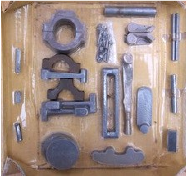
Stuart 5A vertical steam engine casting with reversing gear.
